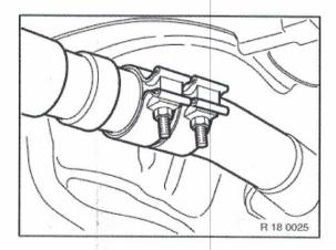
Adjust new rear silencer and connect by clamp to centre silencer.
