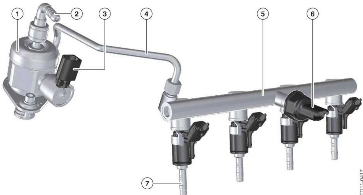
N13 engine, fuel preparation
