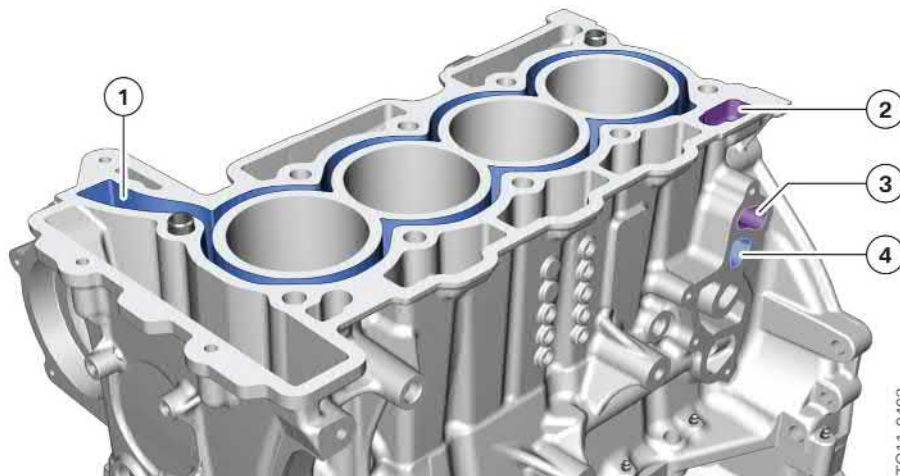
N13 engine, cooling jacket and coolant ducts
