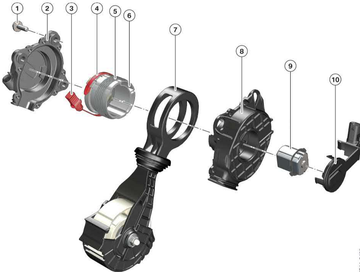
N13 engine, friction gear servodrive - exploded view
