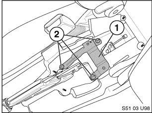
Locate proper position of DSC sensor bracket
