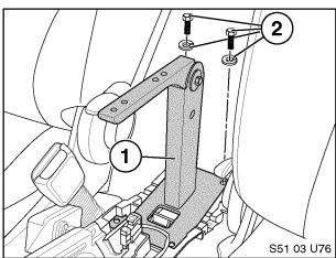
12. Secure armrest base (1) to hex spacers using M6x20mm hex head bolts with M6 split lock washers (2) as shown.
