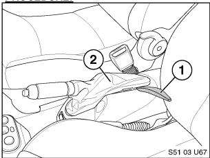
1. Use trim removal tool (1) to carefully pry out handbrake surround trim piece (2) as shown.
