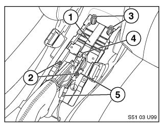
7. Reinstall console support bracket (1). Reinstall front pair M6 nuts (2). Install kit supplied pair of M16x56mm hex standoffs (3) on threaded M6 studs as shown.
