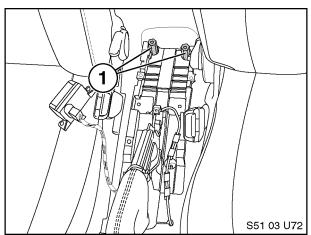
8. Install pair of M16x56mm hex standoffs (1) on threaded M6 studs as shown.
