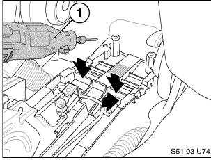
10. Remove any interfering material (black arrows) from console support bracket as necessary by using a Dremel<sup>®</sup> (1) or similar rotary tool with a grinding bit as shown.
