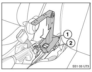
9. Test fit armrest base assembly (1) onto console support bracket (2) to determine where interfering material on console support bracket must be removed to achieve levelness and stationary fit of armrest base assembly.
