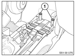
11. Test fit armrest base assembly to console support bracket/hex standoffs assembly for levelness. Install M6 flat washer(s) (1) as shims on top of hex standoff (1) as necessary to achieve levelness.
