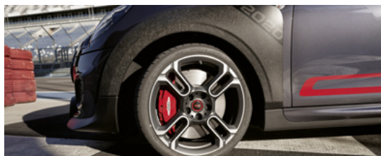
18" forged lightweight wheels with Hankook sport tyres, sport braking system and Carbon fibre individually numbered wheel spats
