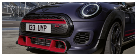
Piano Black Exterior features, front grille insert with honeycomb grille and upper air intake, front bumper with new air intake, Chili Red accents
