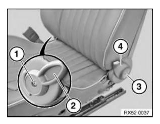
Release Torx screw (1) from lever (2) for backrest angle adjustment.
