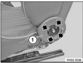
Unclip rear panel (1) on left and right from backrest frame.
