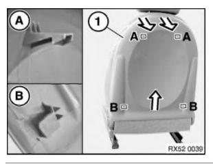
Unclip rear panel (1) from backrest frame in area (A). Remove rear panel (1) in area (B) from backrest frame in upward direction.
