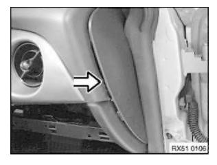
Lever out cover on left and right in direction of arrow.
