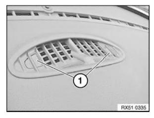
Lever out cover caps (1) in ventilation grille and release screws underneath.
