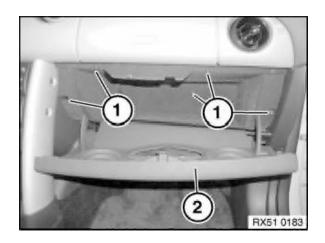
Release screws (1). Remove glovebox (2).
