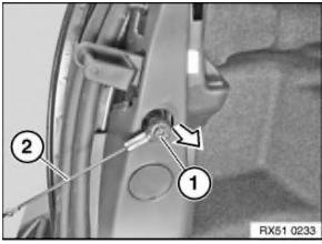
Release screw (1) on retractor Bowden cable (2).
