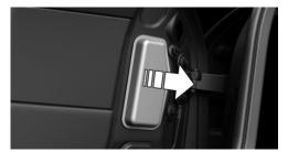
3. Press the latches together upward, arrow 1, and remove the bulb holder.
