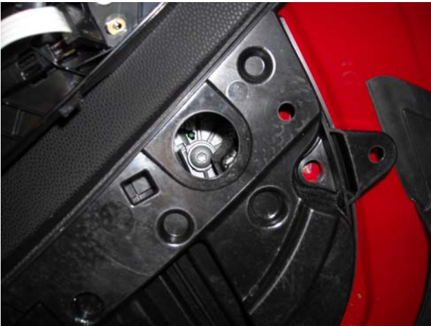
Lower window adjusting height until window glass thru bolt is exposed. This is the rear access hole.
