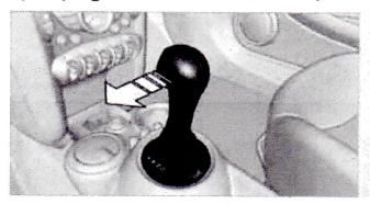
Move the selector lever from position D to the left into the M/S shifting slot:
