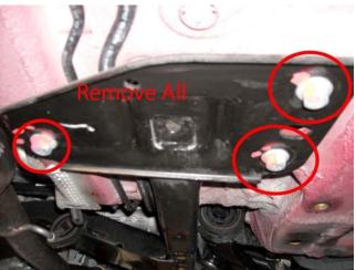
Lower Sub Frame and remove 2 Control Bushing Carrier Mounting Bolts (very tough)
