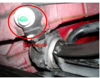
**Remove Motor Mount Attaching Bolt**
