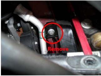
Remove Wishbone / Control Arm Carrier Bolt
