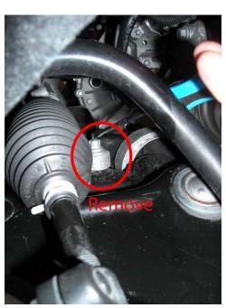
Remove Rear Sub Frame to Bumper Connecting Bolts and Loosen Front Bolts
