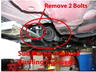
Use 3 Jaw Puller and Remove Control Arm Bushing/Carrier/Wishbone Bracket
