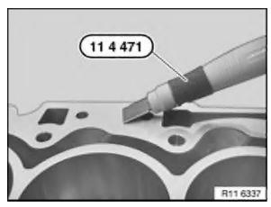
Use special tool 11 4 471 to remove coarse gasket remnants from sealing faces of cylinder head and crankcase.
