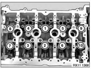
Release cylinder head bolts with special tool 11 2 250 . Release cylinder head bolts from outside inwards (10 to 1).
