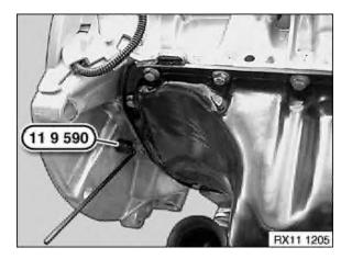
Secure crankshaft with special tool 11 9 590 .
