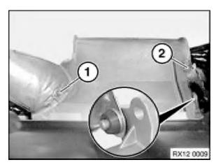
Unscrew bolt (1). Release retaining clip (2). Remove heat shield. Tightening torque 12 41 1AZ .
