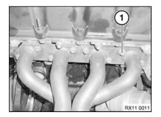
Unscrew 8 retaining screws (1) at exhaust manifold. Remove exhaust manifold.
