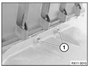
Undo retaining screws (1) for heat shield. Tightening torque 11 62 1AZ .
