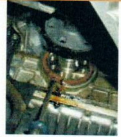
Removing a leaking rear main seal
