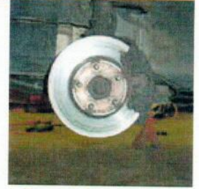
Damaged brake rotor from metal-to-metal contact
