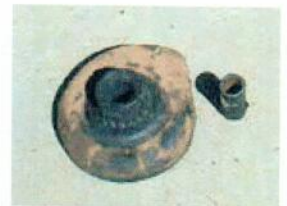
Broken strut mount
