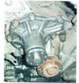
New water pump
